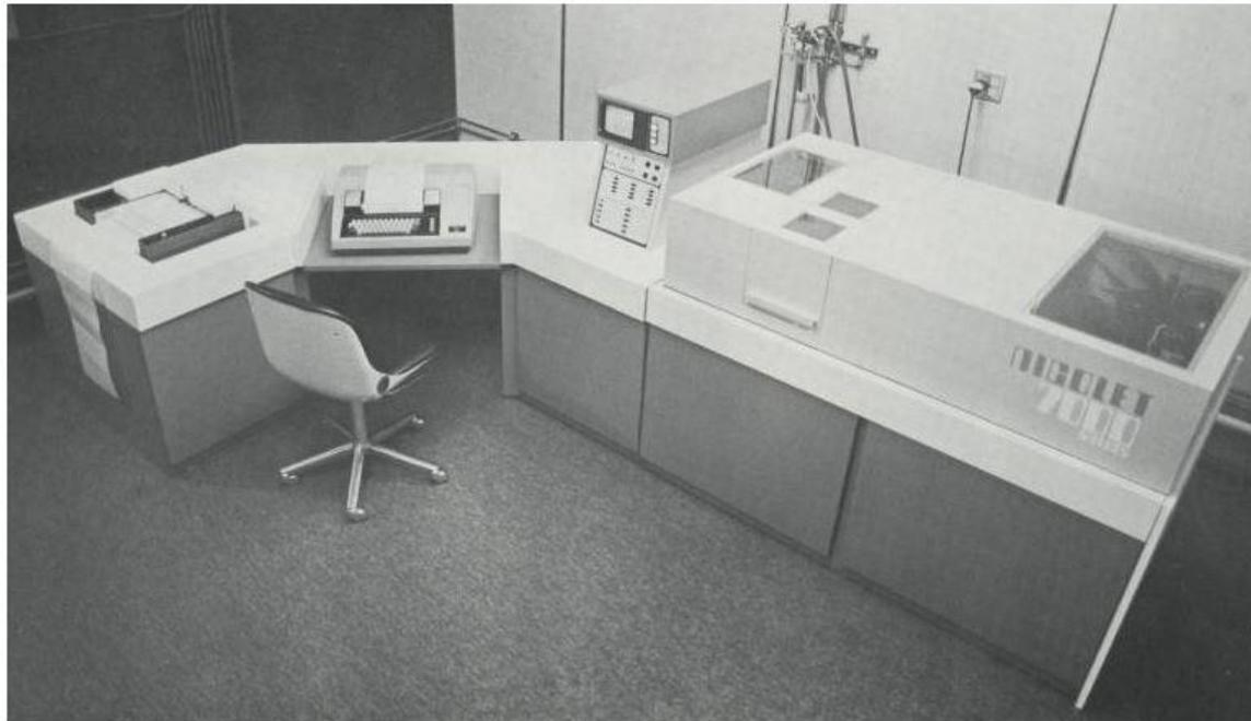
The 7199, introduced in 1977, was Nicolet's first FTIR. The Mini-Cooper sized enclosure was made of chipcore and blue and pale blue Formica. An 1180 hid in it. It was an immediate success. Nicolet became, and still is, the world's largest FTIR company.
