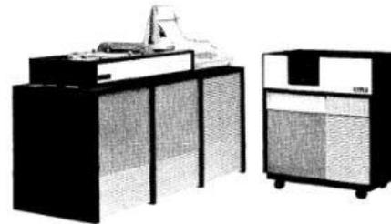
The DIGILAB FTS-14 is the first Fourier Transform infrared spectrophotometer. It uses a large-aperture interferometer and a powerful mini-computer instead of slits, prisms or gratings, and analog circuits.
